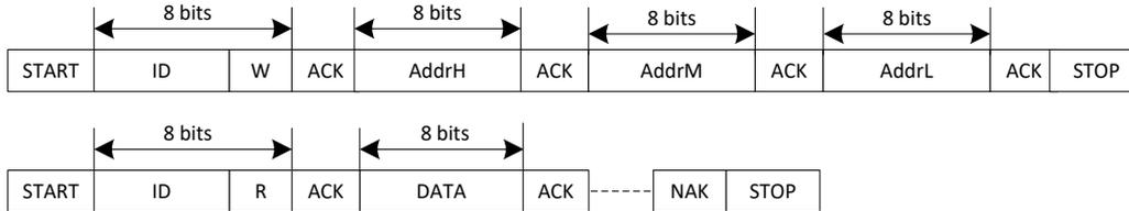
Figure 7- 5 Read format in DMA mode
