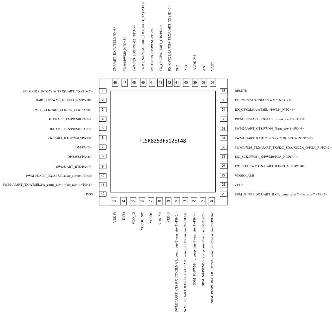
Figure 1- 4 Pin assignment for TSLR8253F512ET48
