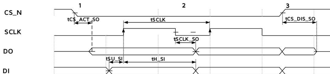
Figure 15- 3 SPI Timing Diagram, Slave Mode
