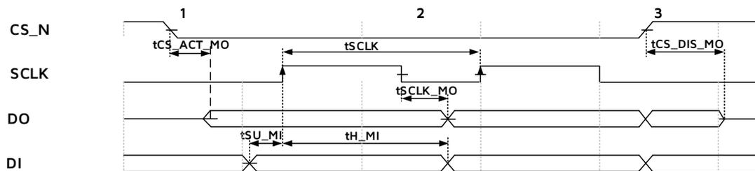
Figure 16- 2 SPI Timing Diagram, Master Mode
