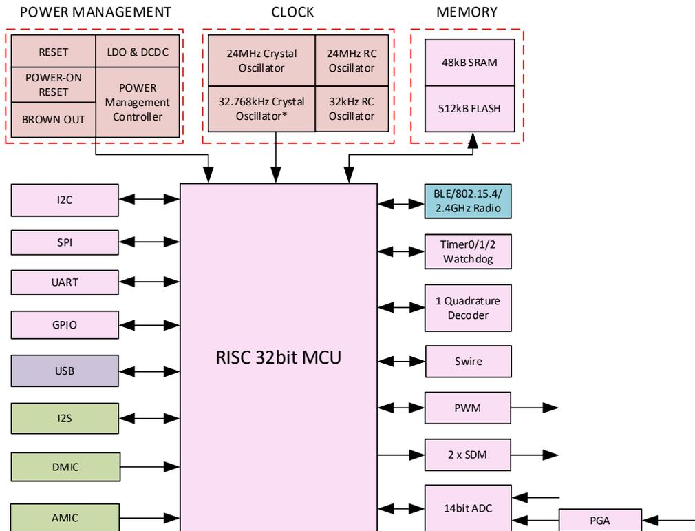
Figure 1- 1 Block diagram of the system
