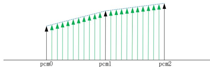
Figure 9- 4 Linear interpolation
