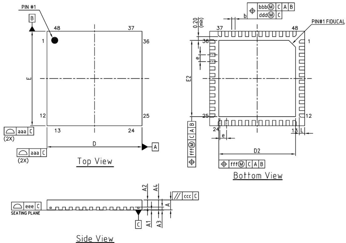
Figure 1- 2 Package dimension for TLSR8253F512ET48 (Unit: mm)
