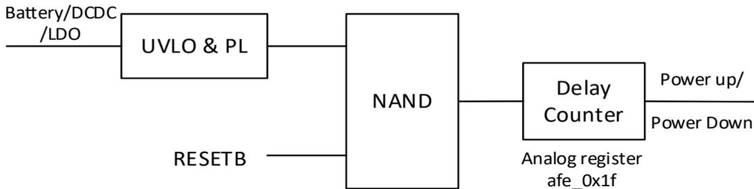
Figure 2-3 Control logic for power up/down
